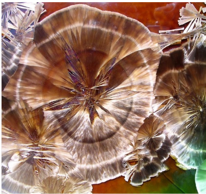
Fig. X.X Some of my favorite crystals, these colored mainly with manganese. The lighter-colored "growth rings" were made during a cooling cycle, and the darker ones during a heating cycle. This is typical—but not guaranteed—of efforts to grow such rings.
