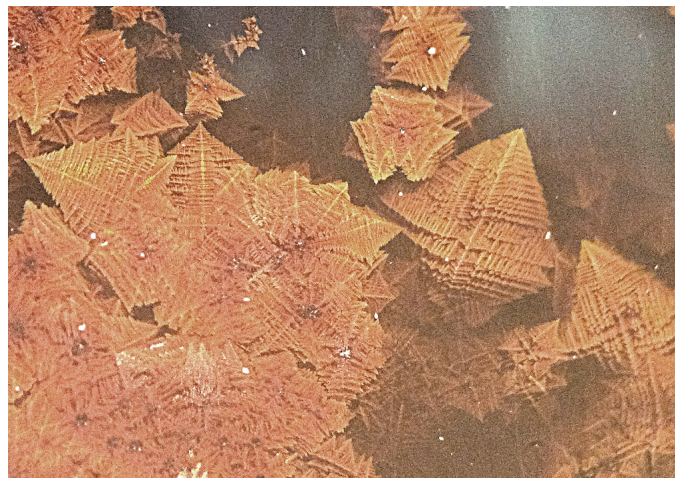
Fig. X.X. Pyramids of cristobalite growing in a high-iron, high-titanium glaze.
