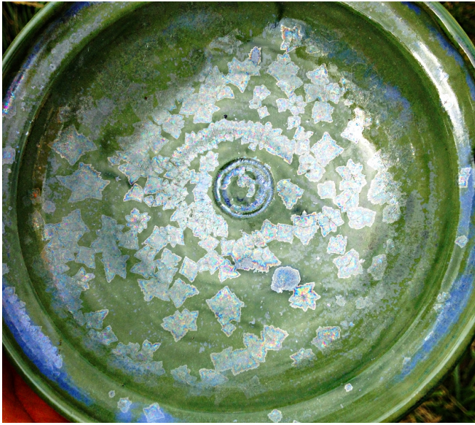
Fig. 4.X. Copper carbonate, and perhaps a touch of chrome, in a molybdenum glaze.
