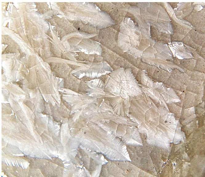
Fig. 5.3. Transparent sphene and wollastonite crystals.
