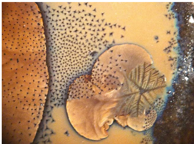
Fig. X.X. A flock of partially-submerged hatrurite crystals, with a zince silicate and a trööstite crystal thrown in for good measure. The triangular shape is indicative of hatrurite. Compare these with the hexagonal stars of fayalite, below. Photo: Evan Cornish-Keefe.
