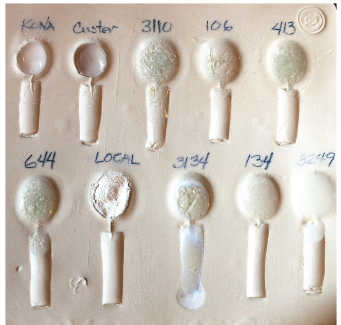
Fig. 3.x. Drip Test Tile, comparing two commercial feldspars, one badly-prepared local feldspar, and six frits, on Laguna’s 631 Porcelain.
