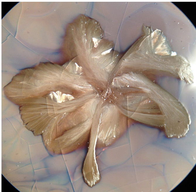
Fig 1.3. As fine an example of cyclic twinning as you're going to see in a glaze. Wollastonite crystals grown by Evan Cornish-Keefe, 10x magnification.
