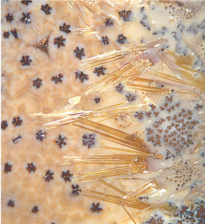
Fig X.X. Fayalite stars. This hexagonal twinning is the norm for fayalite in a glaze. Also visible are cristobalite and rutile crystals.
