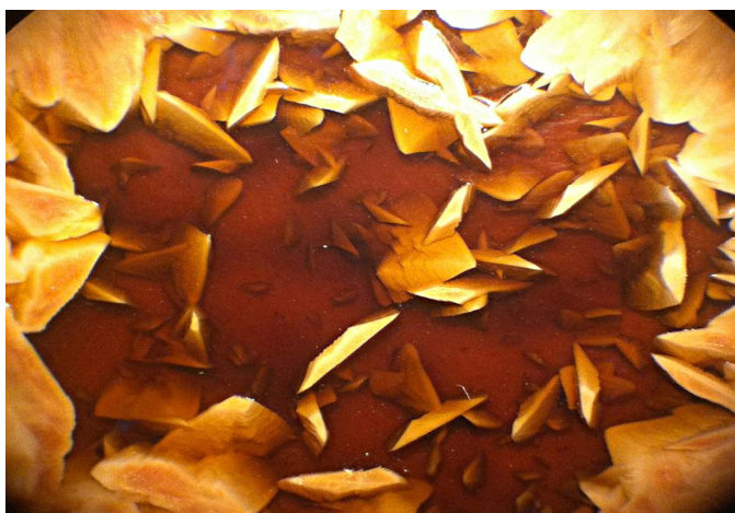
Fig 5.2. Sphene crystals in a pool of glaze, showing the characteristic shape of sphene crystals as they grow in nature.
