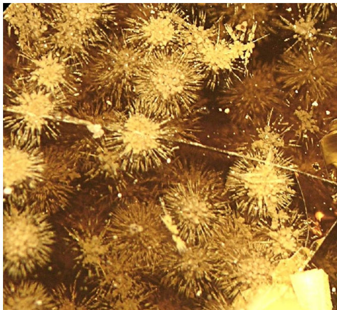
Fig X.X. Tridymite prefers to grow in overlapping plates, in both nature and in glazes.
